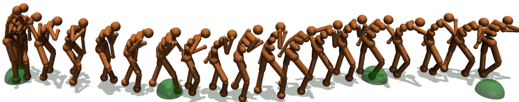
Figure 1: A humanoid agent discovers diverse locomotion primitives without any reward using DADS. We show zero-shot generalization to downstream tasks by composing the learned primitives using model predictive control, enabling the agent to follow an online sequence of goals (green markers) without any additional training.
