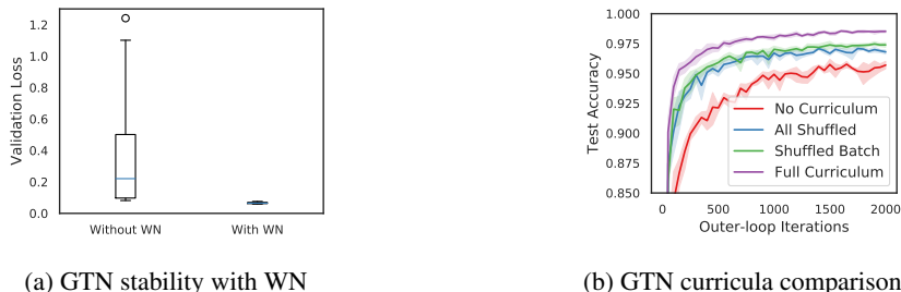
Figure 2: Both a learned curriculum and weight normalization substantially improve GTN performance. (a) Weight normalization improves meta-gradient training of GTNs, and makes the method much more robust to different hyperparameter settings. Each boxplot reports the final loss of 20 runs obtained during hyperparameter optimization with Bayesian Optimization (lower is better). (b) shows a comparison between GTNs with different types of curricula. The GTN method with the most control over how samples are presented performs the best.
