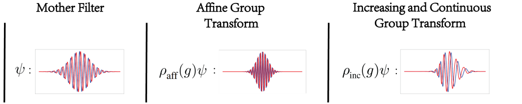
Figure 3: Transformation of a Morlet Wavelet: For all the filters, the real part is shown in blue and the imaginary in red. (left) Morlet wavelet mother filter. (middle) Transformation of the mother filter with respect to the affine group: the parameters of the group are 0 < a < 1 , i.e., contraction, and b = 0 , i.e., no translation. (right) Increasing and continuous group transformation of the mother filter for some randomly generated function g \in \mathbf{G}_{\text{inc}} leading to chirp-like transform.
