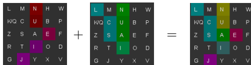
Figure 2: Comparison of two strings. To compare the names “JEN” and “LIN”, we add the string-map for “JEN” (left image) to the string-map for “LIN” (middle image) to generate the final comparison image (right image).
