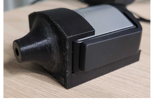
Figure 1: Colorimeter used to tune colour appearances between the Hololens 2 and the opaque display with its 5mm aperture attachment, allowing us to take contact measurements on the Hololens 2 displays.
