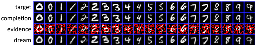
Figure 4: MNIST completions. Row 1: target test examples, with class label coded in the bottom row. Row 2: completions produced by the FBAN. Row 3: Evidence with masked regions (including class labels) in red. Row 4: the top-down ‘dream’ state produced by the hidden representation.
