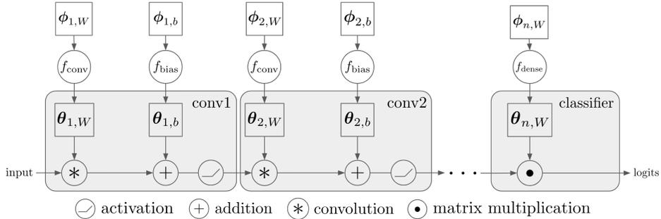
Figure 2: Classifier architecture. The  $\phi$  tensors are stored in their compressed form. During inference, they are read from storage, uncompressed, and transformed via  $f$  into  $\theta$ , which are then used as parameters in typical convolutional or dense layers. When uncompressed,  $\phi$  are integer tensors.
