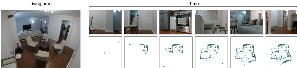
Figure 4: Real-world Transfer. Left: Image showing the living area in an apartment used for the real-world experiments. Right: Sample images seen by the robot and the predicted map. The long-term goal selected by the Global Policy is shown by a blue circle on the map.
