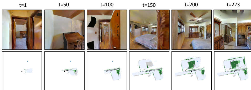
Figure 9: Pointgoal visualization. Figure showing sample trajectories of the proposed model along with predicted map in the Pointgoal task as the episode progresses. The starting and goal locations are shown by black squares and blue circles, respectively. Ground truth map is under-laid in grey. Map prediction is overlaid in green, with dark green denoting correct predictions and light green denoting false positives. Blue shaded region shows the explored area prediction.
