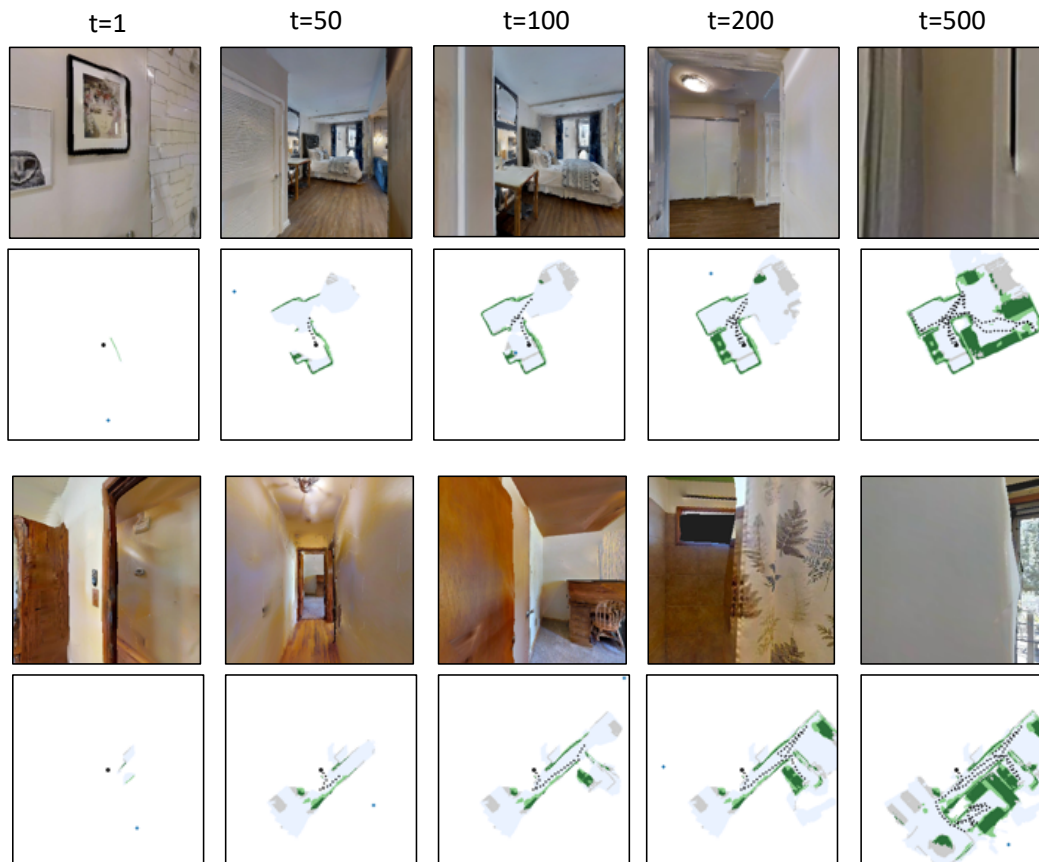
Figure 8: Exploration visualization. Figure showing sample trajectories of the proposed model along with predicted map in the Exploration task as the episode progresses. The starting location is shown in black square. Long-term goals selected by the Global policy are shown by blue circles. Ground truth map is under-laid in grey. Map prediction is overlaid in green, with dark green denoting correct predictions and light green denoting false positives. Blue shaded region shows the explored area prediction.
