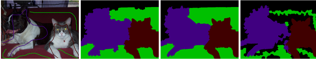
Figure 1: Left: image with scribbles from Pascal VOC dataset. Mid-left: semantic segmentation result of our heuristic with layer 3 of ResNet 101. Mid-right: result of our ILP with probability map of DeepLab V2. Right: ILP without connectivity prior (with DeepLab V2 prob. map).
