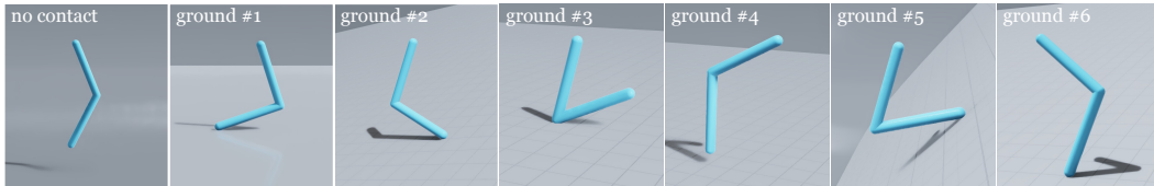
Figure A.1: Seven Double Pendulum contact configurations used for testing NeRD 's generalizability across different contact environments.
