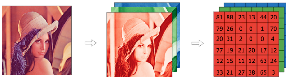
Figure 3: RGB decomposition, a colored image is a 3-tensor.
