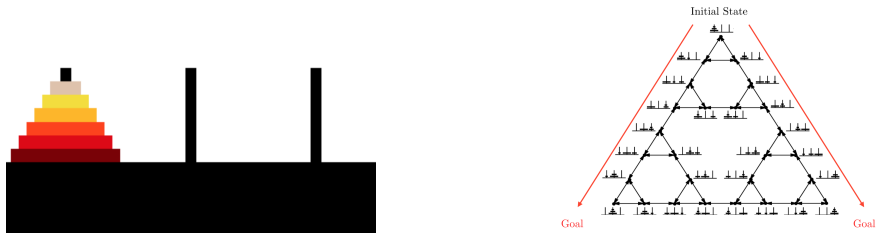
Figure 5: (Left) The Tower of Hanoi. (Right) State space for the three disk problem.
