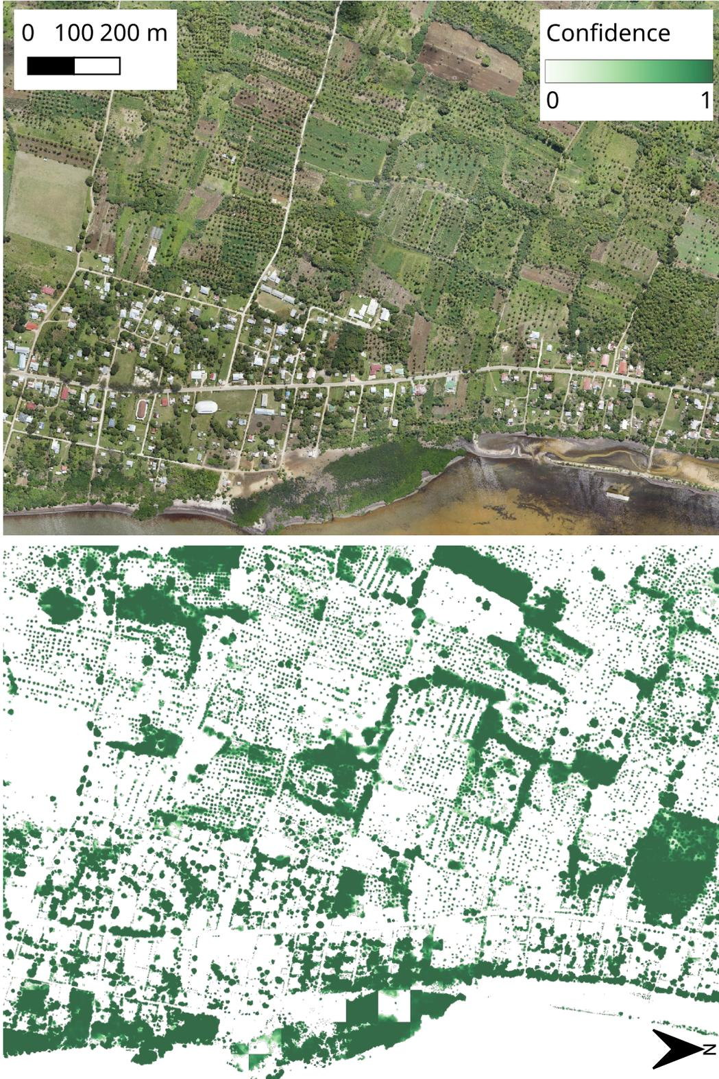
Figure 7: Semantic segmentation predictions for the WeRobotics Open AI challenge image over the Kingdom of Tonga, using the `restor/tcd-segformer-mit-b5` model. Individual palm trees are clearly segmented. Some uncertain predictions are visible in the lower region of the image near the coast - identifiable as missing/inconsistent tiles.
