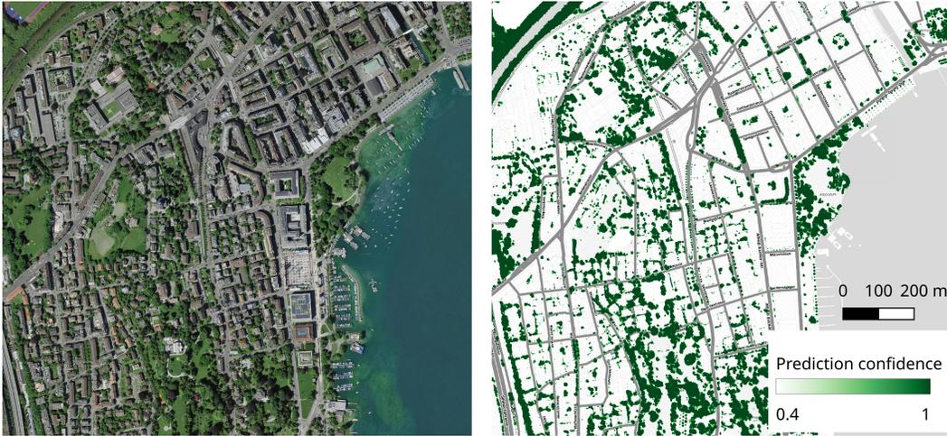
Figure 1: Tree semantic segmentation for Zurich, predicted at 10 cm/px. Predictions with a confidence of  $< 0.4$  are hidden. Left: 10 cm RGB orthomosaic provided by the Swiss Federal Office of Topography swisstopo/SWISSIMAGE 10 cm (2022), Right: prediction heat map. Zooming in is recommended to see small details, e.g. trees along the top edge of the lake. Base map tiles by Stamen Design, under CC BY 4.0. Data by OpenStreetMap, under ODbL.
