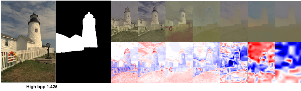
Figure 27: Reconstruction and visualization of latents for kodim-19 at high (1.425 bpp) bitrates. The first row shows reconstructions with only one of seven latent modulation sets active at a time. The second row visualizes the corresponding raw latents, upsampled to output resolution.
