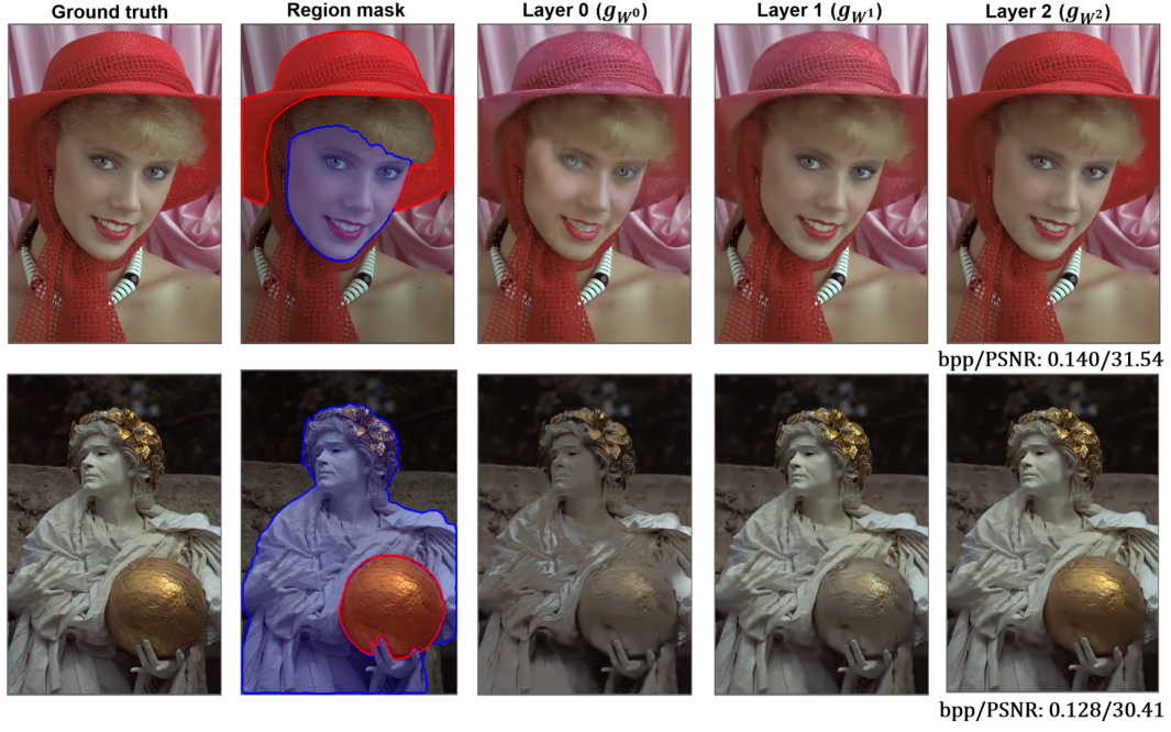
Figure 28: Visualization of layered compression: The background LSN g_{W^0} is first transmitted as layer 0, followed by g_{W^1} for the blue region (layer 1), and finally g_{W^2} for the red region (layer 2). We can see that colors and textures (e.g., red hat and golden ball) are refined with the additional LSN parameters.
