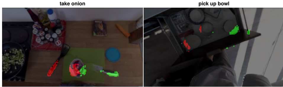
Figure 7: Failure cases. In both cases the model is undecided of what to do. In the left example it predicts affordance regions at different objects that are also not related to the task, i.e., the spatula and the knife. In the right example the model predicts a bimanual action to pick up the bowl and predicts affordance regions at multiple bowls even though only one bowl is supposed to be picked up.
