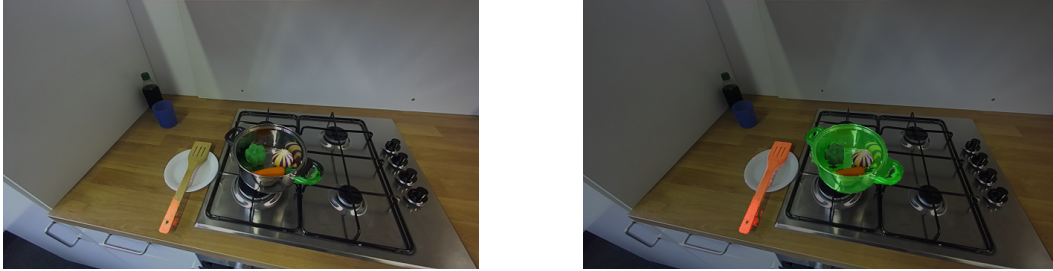
Figure 9: The affordance detection of our method detects precise affordance regions (left) for the pot and the spatula that can be used to successfully perform the task of stirring within the pot. The right image shows the mask outputs by LangSAM. The text prompts used for this prediction were “wooden spatula” and “cooking pot” for LangSAM and “stir vegetables” for 2HandedAfforder.
