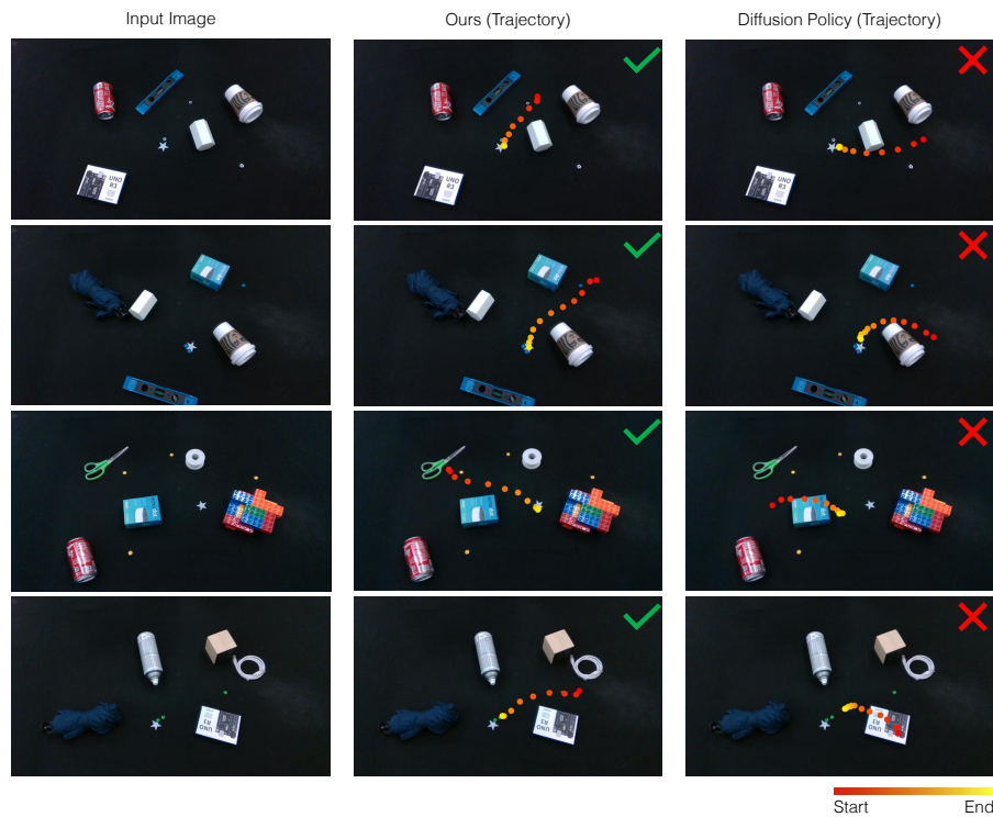
Figure 3: Additional Sweeping Qualitative Results. The trajectory of the end-effector is projected onto the input image.
