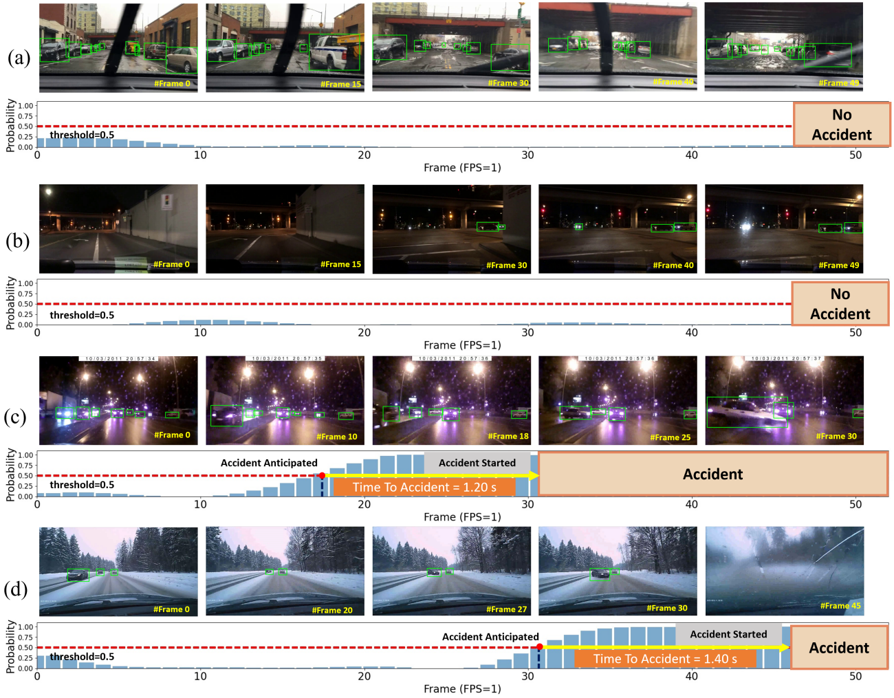
Figure 2: Qualitative Results of the CRASH on the CCD dataset: (a) and (b) depict scenarios without accidents, while (c) and (d) illustrate scenarios with accidents. The blue bars represent the model’s output of the probability of an accident occurrence, with the threshold uniformly set at 0.5
