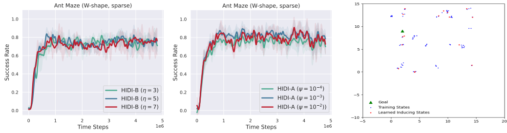
928 Figure 4: (Left) Impact of \eta , which balances the diffusion objective and RL objective. (Middle) Impact of \psi , 929 which adjusts the influence of GP prior in learning the distribution of diffusional subgoals. (Right) Visualization 930 of the learned inducing states (2D coordinates) compared with the complete training data.
