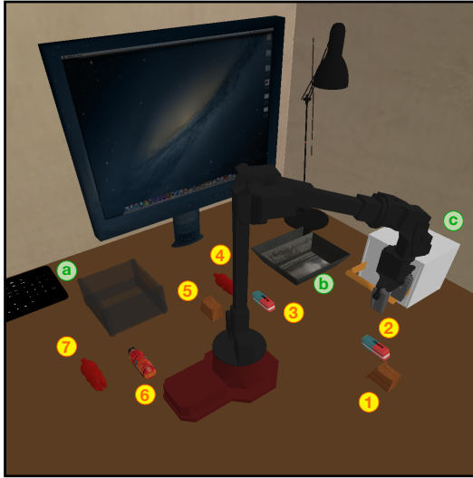
Figure 10: Office cleanup task. The robot agent needs to place three randomly sampled objects (1-7) inside randomly sampled containers (a-c). During task-agnostic data collection we apply random noise to the initial position of the objects.
