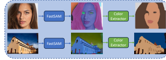
Figure 14: Palette generation pipeline. First, we employ FastSAM (Zhao et al., 2023b) to segment the image. Then, we get the dominant color for each segment.
