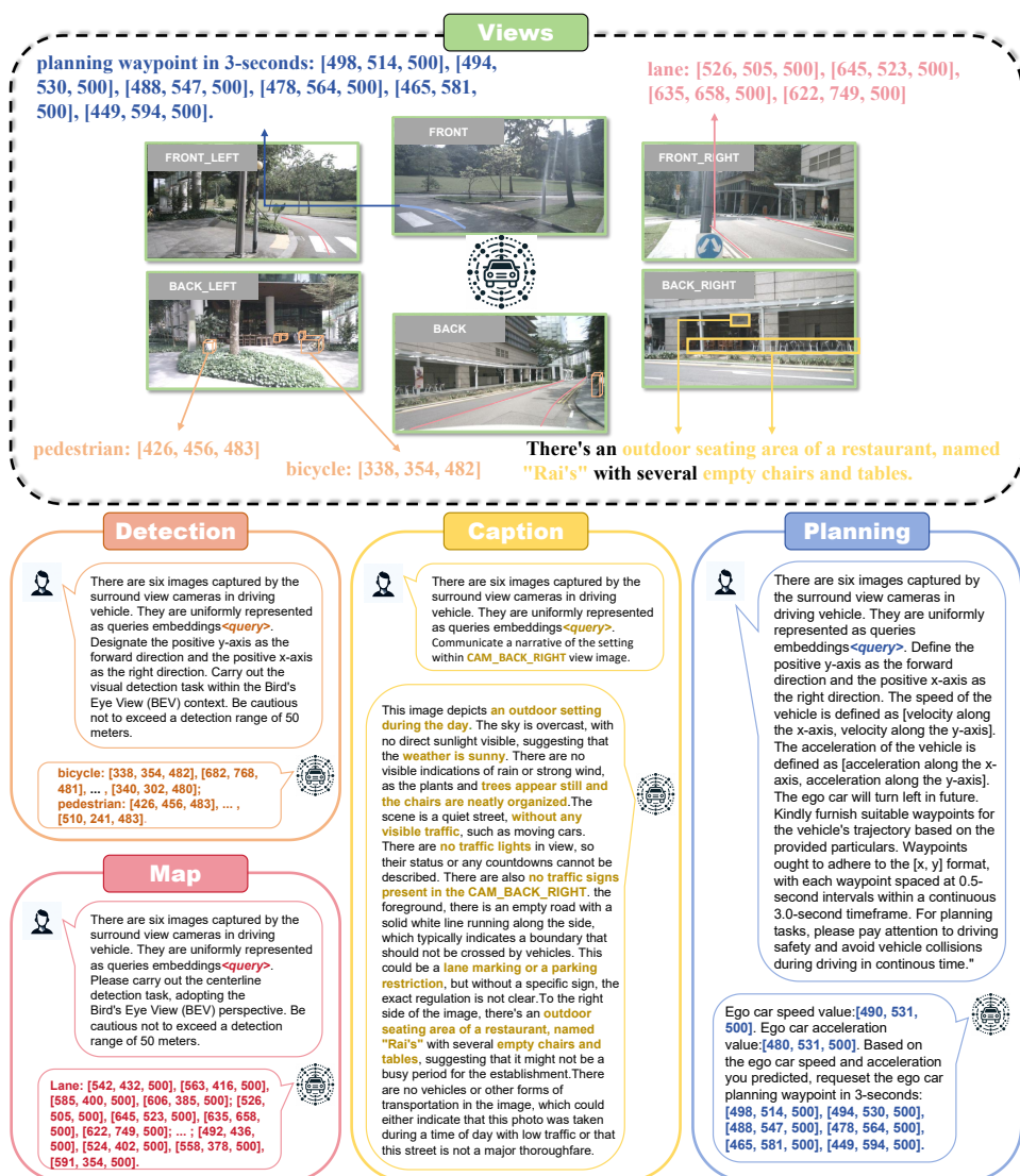
Figure 1: Our constructed question-answer pairs for VLM-based methods. It transforms several critical driving reasoning tasks, such as 3D object detection, map perception, environment caption, and ego-car planning, into a uniform text format.
