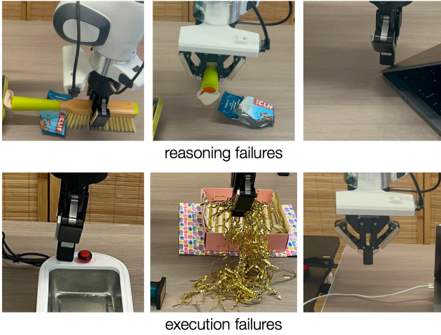
Fig. 5: Failure analysis. We breakdown the failure cases of the variants of our approach using zero-shot prediction, distilled policies, and in-context learning. We breakdown the failures into reasoning failures (caused by errors in the affordance prediction) and execution failures (caused by low-level motions).
