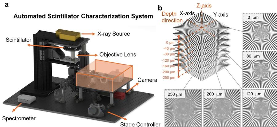
Fig. A.1 X-ray Imaging Data Acquisition System. (a) In-situ depth-scanning data acquisition setup. (b) Z-stack microscopic imaging of the scintillator under X-ray excitation.
