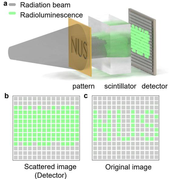
Fig. 1: Schematic of X-ray imaging. (a) A general radiation imaging system. (b, c) Comparison of scattered and original images.
