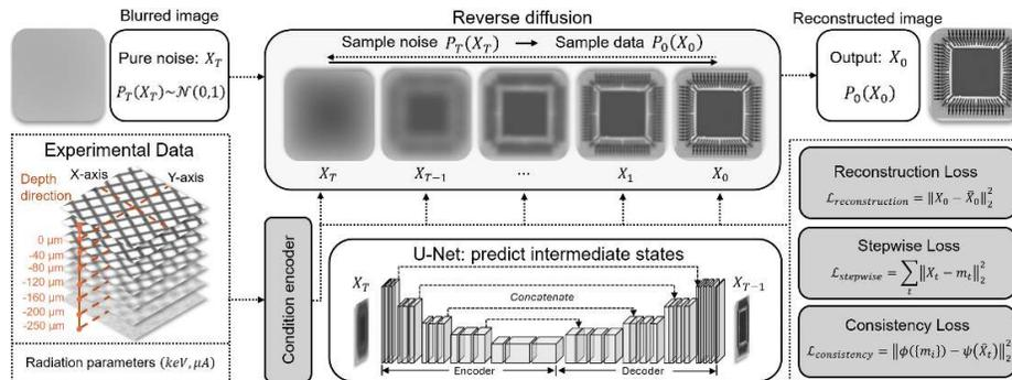
Fig. B.1 Scattering-aware diffusion model for image reconstruction. Using a continuous conditional diffusion model constrained by actual diffusion images from our own data collection platform and has high image restoration fidelity.
