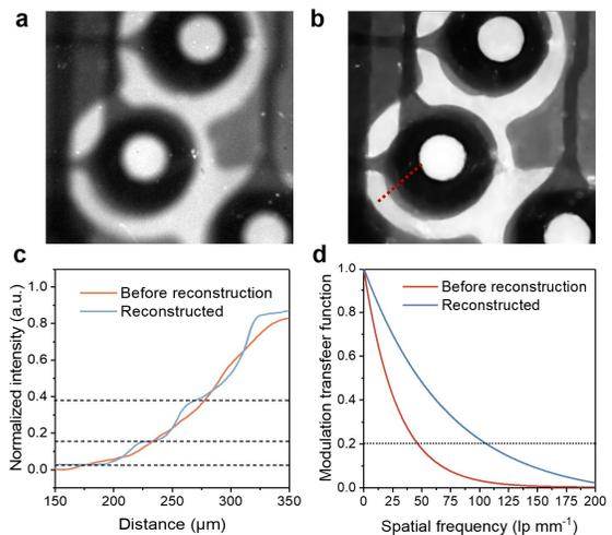
Fig. 2: Reconstruction of X-ray images of circuit board chips. (a) Raw detector image. (b) Reconstructed image. (c) Contrast comparison. (d) Resolution comparison.
