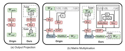
Figure 5: Fusing smooth parameters into the Mamba structure.
