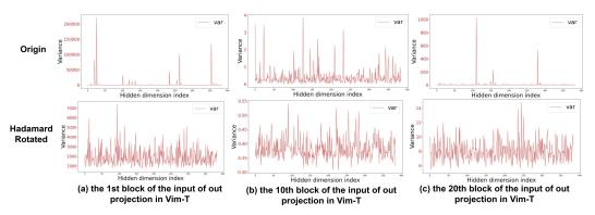
Figure 9: Variances of input of output projection layer blocks in Vim-T: unequal across channels preand post-Hadamard rotation
