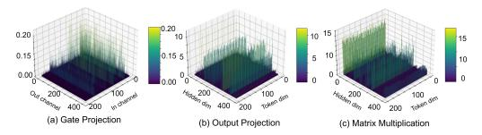
Figure 1: Visualized distribution of hard layers for Mamba quantization. (a) denotes the weight of the gate projection, (b) denotes the input activations of the output projection. (c) represents the output of the parallel scan (PScan) operator, which is also one of the input to the matrix multiplication.
