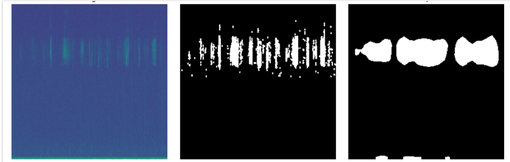
Figure 5: Spectrogram (left), high-quality segmentation mask (middle), and generated pseudo-attention mask (right) for a recording of porpoise clicks.
