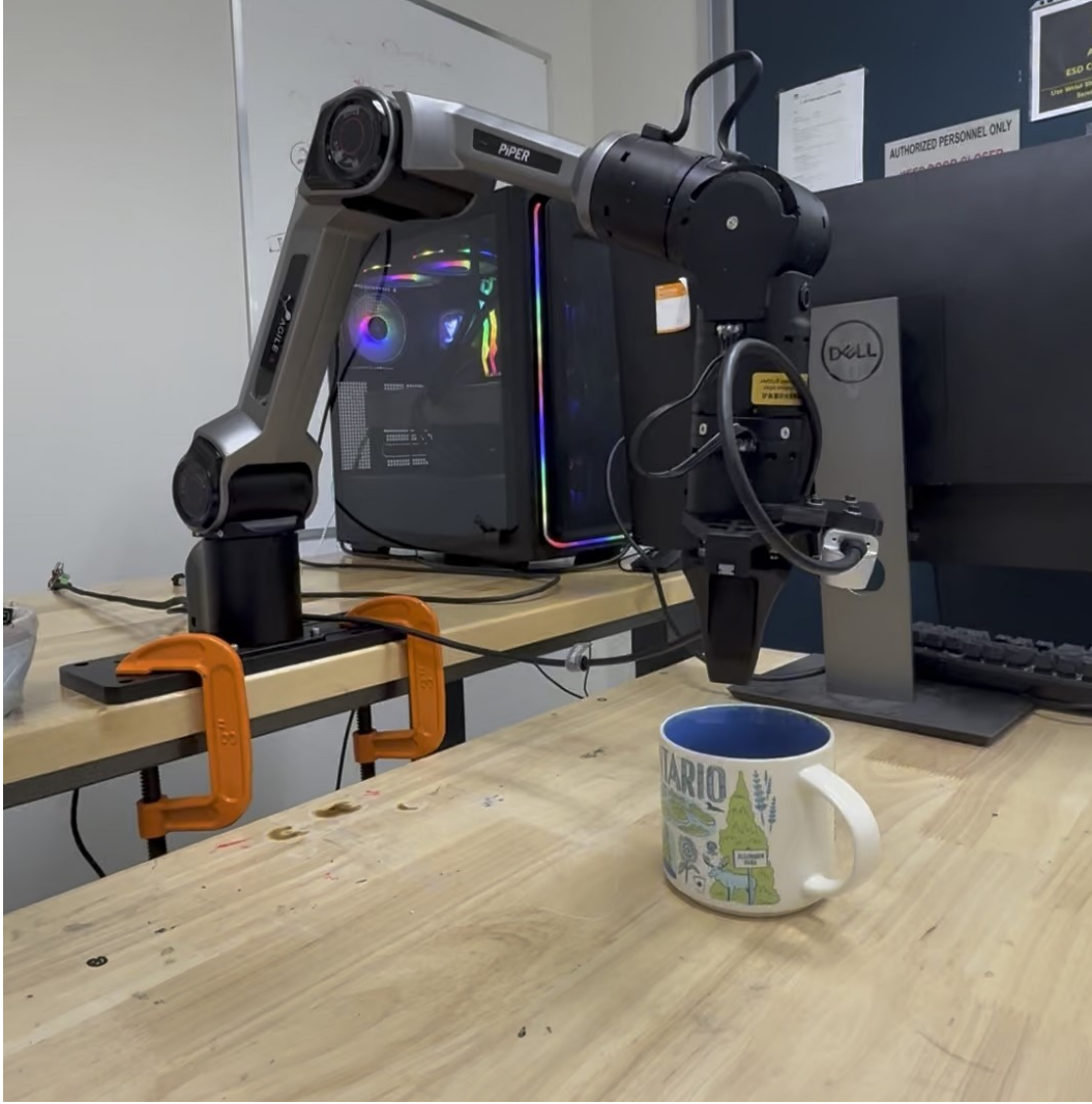
Figure 4: Visualization of UnPose for a real-world robotic manipulation task where it estimates the complete geometry and 6D pose of the cup.
