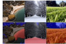
Figure C.4. FG/BG segmentation of classes of water , snow and grass . The foreground is in red, while the background is shown in blue.
