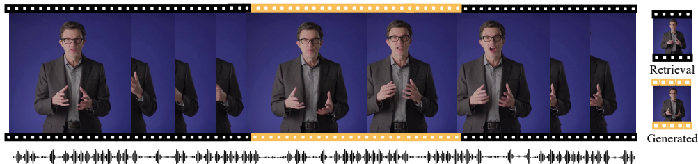
Figure 1: TANGO is a framework designed to generate co-speech body-gesture videos using a motion graph-based retrieval approach. It first retrieves most of the reference video clips that match the target speech audio by utilizing an implicit hierarchical audio-motion embedding space. Then, it adopts a diffusion-based interpolation network to generate the remaining transition frames and smooth the discontinuities at clip boundaries.
