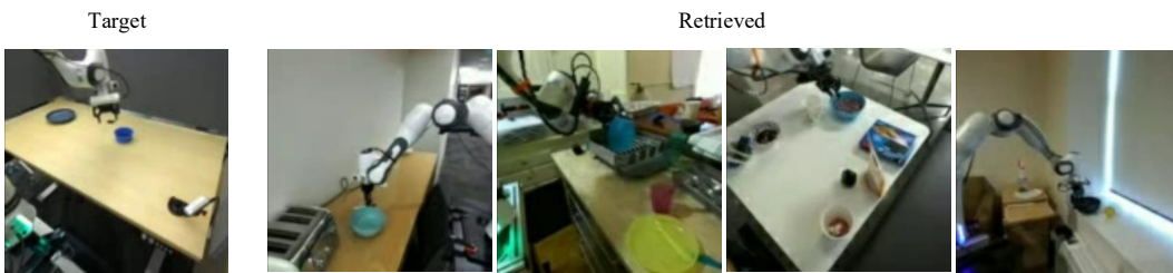
Figure 12: Retrieved cotraining demos for the pour task with the object texture aligned. The camera poses and spatial locations of the target object are not the same, but the color is aligned.
