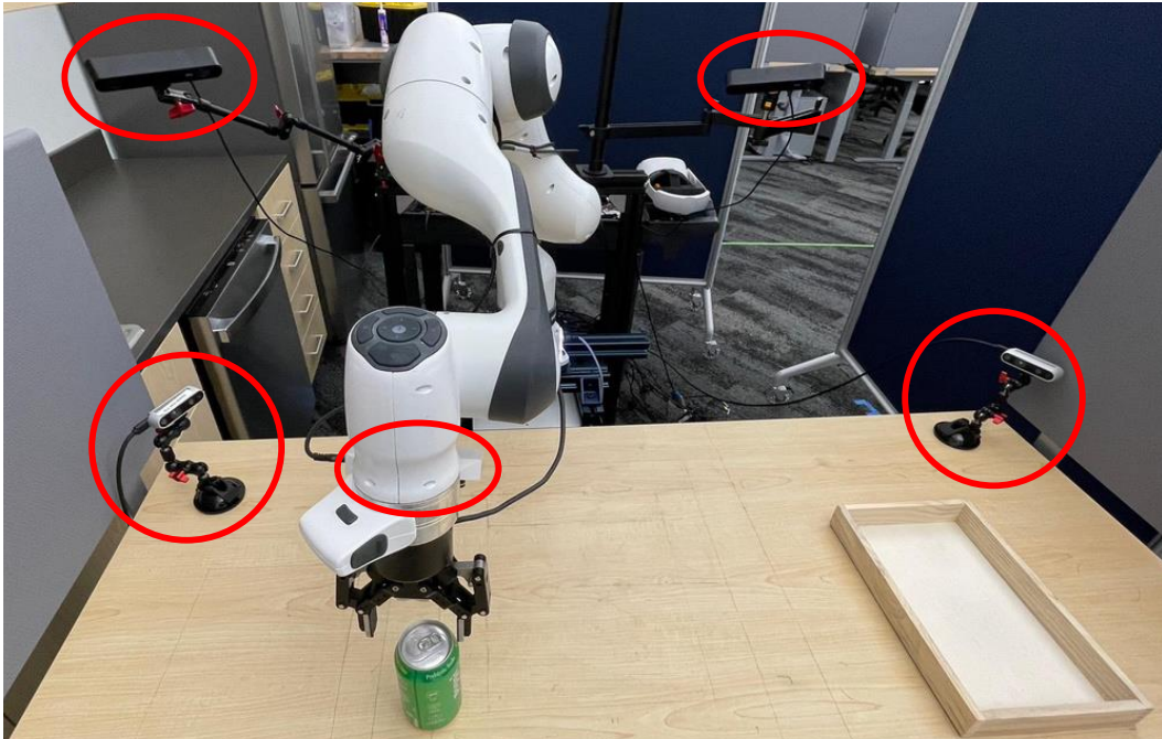
Figure 9: Hardware setup. The red circles show the camera set-up in the real experiment.
