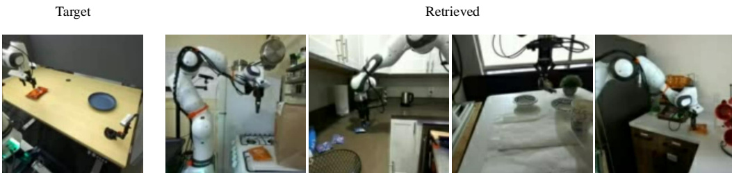
Figure 11: Retrieved cotraining demos for the serve snack task with the object spatial location aligned. The camera poses and textures seen in the demos are not the same as our target task, but the location of the object (in front of the robot and level with its base) is similar.
