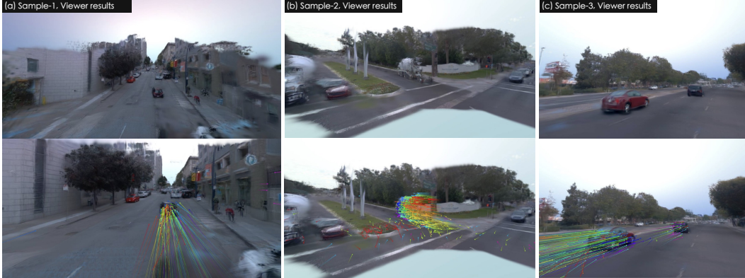
Figure 5: Iterative reconstruction of dynamic scenes. Top: STORM reconstructs 20-second-long videos within 1 second in an iterative manner. Bottom: Furthermore, by chaining scene flows, we obtain point trajectories for dynamic Gaussians.
