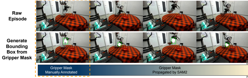
Figure 5: Raw frames (top) are paired with gripper masks (bottom), initially annotated manually (see orange box) and then propagated using SAM2 [84]. Bounding boxes derived from the masks are used for fine-tuning Grounding DINO [70].
