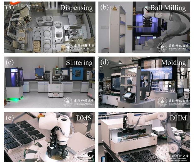
Fig. 2: Automated workstations for energy storage ceramic experiments: (a) Dispensing; (b) Ball Milling; (c) Sintering; (d) Molding; (e) DMS; (f) DHM.
