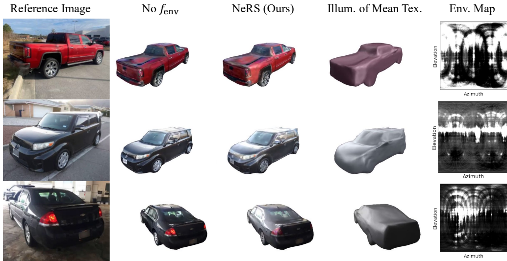
Figure 2: Comparison with NeRS trained without view dependence. Here we compare the full NeRS (column 3) with a NeRS trained without view dependence by only rendering using f_{\text{tex}} without f_{\text{env}} (column 2). We find that NeRS trained without view-dependence cannot capture lighting effects when they are inconsistent across images. The difference between NeRS trained with and without view-dependence is best viewed in video form. We also visualize the environment map and the illumination of the car with the mean texture. The environment maps show that the light is coming primarily from one side for the first car, uniformly from all directions for the second car, and strongly front left for the third car. [Video]
