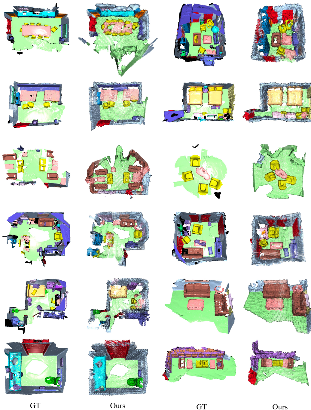
Figure a.13: Qualitative results of semantic segmentation on PeRFception-ScanNet dataset. (1st, 3rd columns) Ground truth point cloud with ground truth semantic labels, (2nd, 4th columns) Reconstructed sparse voxels with predicted semantic labels
