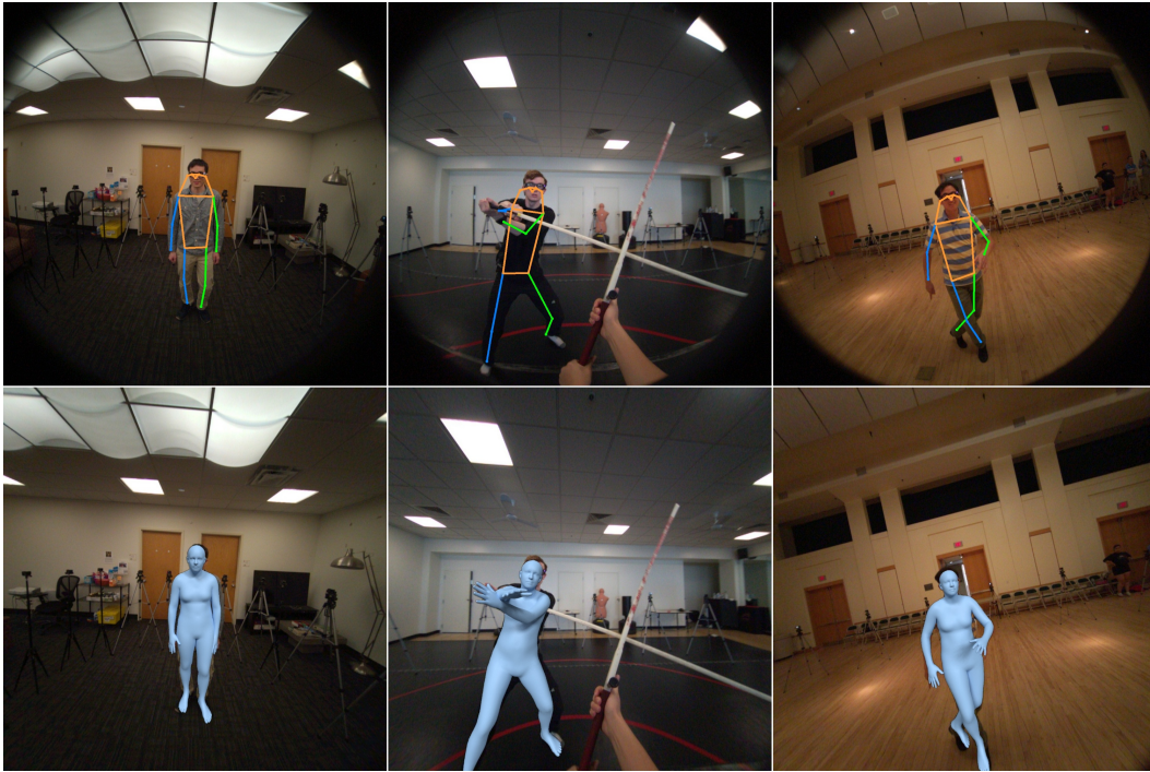
Figure 3: Example of our annotations on the ego-centric images for hugging, fencing, and dancing sequences. The ego-centric image is captured by Meta's Aria glasses. The first row shows the 3D pose, and the second row displays the human mesh.
