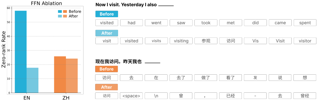
Figure 5: Illustration of the effects of late feed-forward layers ablation (layer 20-23). Left: Zero-rank rate changes comparison between English and Chinese past tense task. Right: Top predicted tokens comparison for before and after ablation. We observe that English performance is significantly impacted after ablation but Chinese is barely influenced. Qualitative results on the right show that the correction token move backward in English but remain the top prediction in Chinese.
