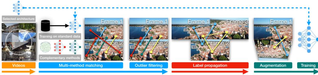
Figure 2: **GIM framework.** We start by downloading a large amount of internet videos. Then, given a selected architecture, we first train it on standard datasets, and generate correspondences between nearby frames by using the trained model with multiple complementary image matching methods. The self-training signal is then enhanced by 1) filtering outlier correspondences with robust fitting, 2) propagating correspondences to distant frames and 3) injecting strong data augmentations.
