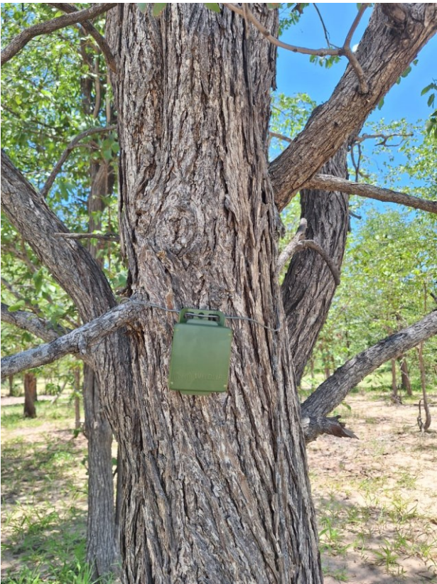
Fig. 1: Acoustic sensor on the tree in MyTree reservation in Chirundu, Zimbabwe
