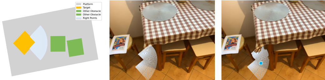
(a) Top-view occupancy map with the target’s right-side search area (b) Sampled points projected onto the 2D image (c) Visible points with the final placement center
