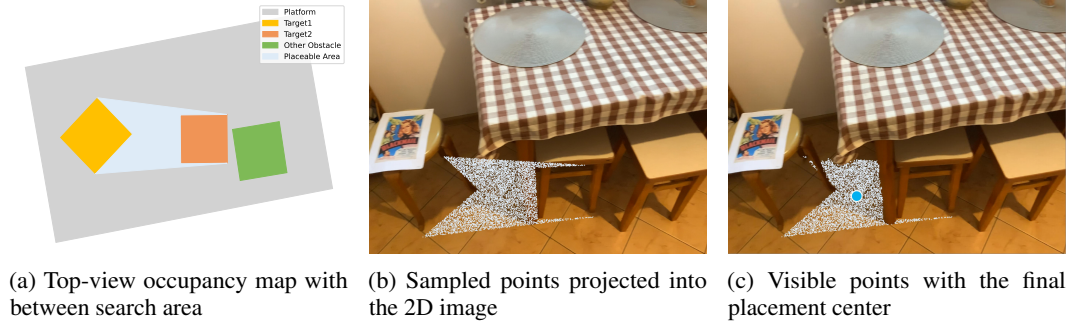
Figure 13: Visualization of between -object free space identification. (a) Top-view occupancy map showing the area between two target objects on the same platform. (b) Projection of sampled points into the image plane. (c) Non-visible points are filtered; the final placement center is indicated.
