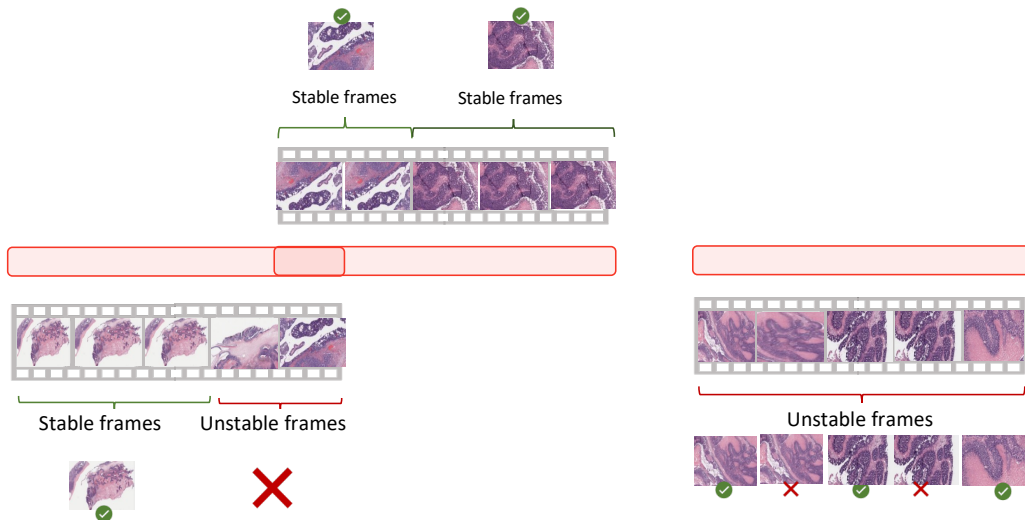
Figure 2: Representative Frame Identification. If a Stable frame is found by Algorithm 1 within the candidate regions, we use it as the representative frame. If not, we use the most dissimilar frames among unstable frames.
