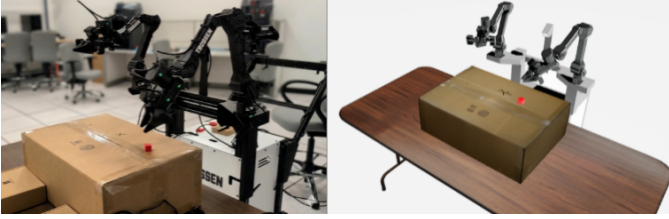
Fig. 2: Qualitative visual comparison between real environment (left) and reconstructed digital twin (right). The twin preserves key scene features including object layout, geometry, and surface texture.
