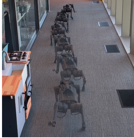
Figure 6: Real-World Deployment. Frame overlay demonstrating the deployment of the BoT walking policy to a Unitree A1 quadruped robot.
