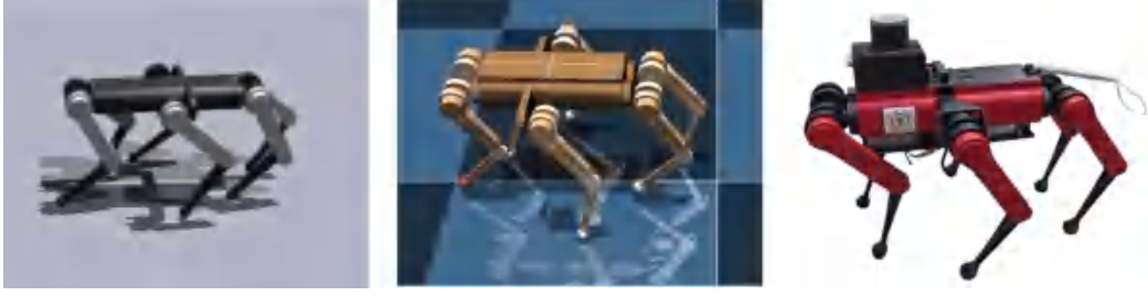
Figure 8: Custom-built hexapod robot in Isaac Gym, MuJoCo, and the real world.
