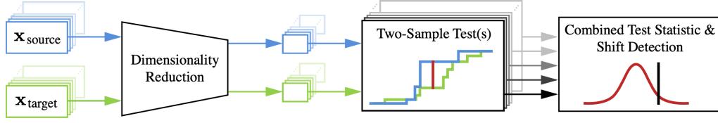
Figure 3: The procedure of detecting a dataset shift using dimensionality reduction and then a two-sample statistical test. The dimensionality reduction is applied to both the detection-training (source) and test (target) data, prior to being analyzed using statistical hypothesis testing. This figure is taken from [10].
