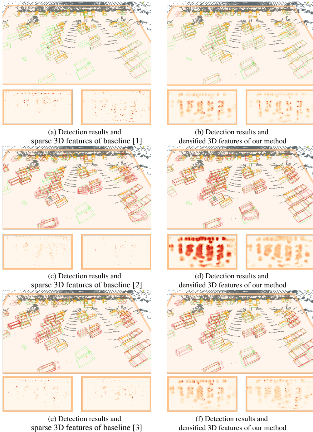
Figure A2: Visual comparison of 3D object detection results and 3D features produced by (a,c,e) baselines [1–3] and (b,d,f) our methods (our approach + corresponding baseline), where our approach successfully densifies the object features and helps the baseline methods produce more accurate detection results than three baselines. Note that red boxes show the detection results and green boxes show the ground truths. Orange boxes highlight the improvement brought by our approach.
