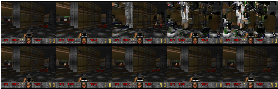
Figure 4: Auto-regressive drift. Top: we present every 10th frame of a simple trajectory with 50 frames in which the player is not moving. Quality degrades fast after 20-30 steps. Bottom: the same trajectory with noise augmentation does not suffer from quality degradation.
