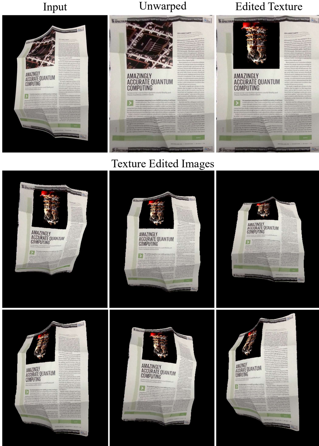
Figure 17: Example of texture edited images from different views. Note the perspective changes and deformation on the edited texture due to the complex shape of the paper.
