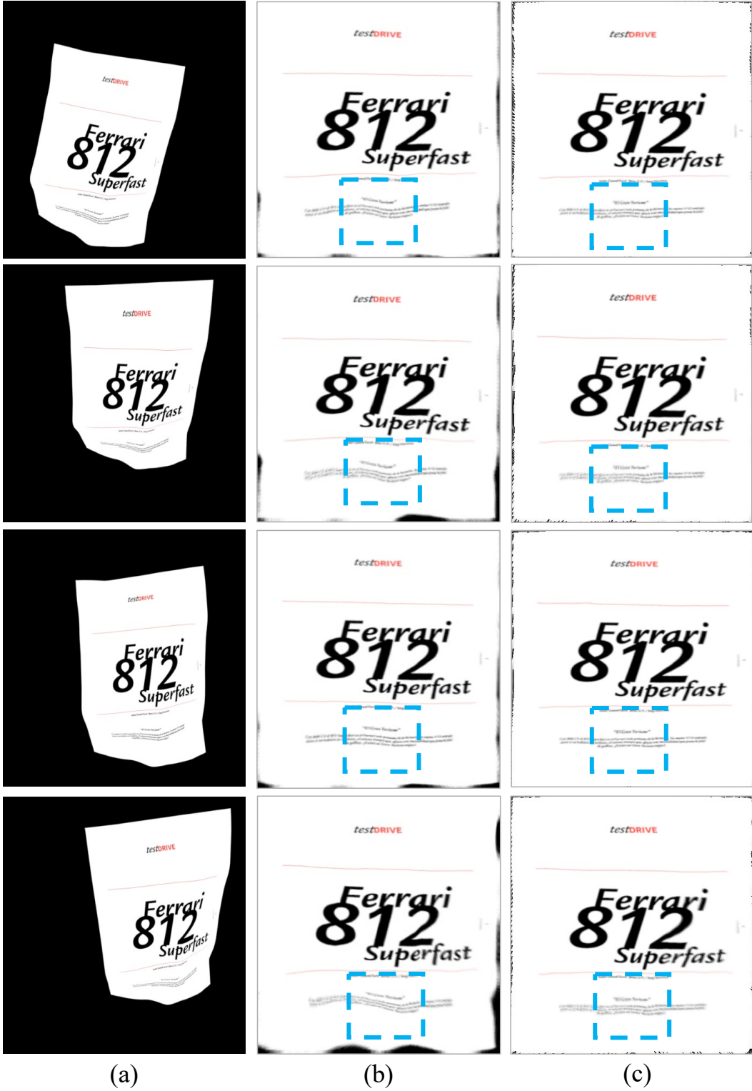
Figure 8: 4 best results (sorted in ascending order from top to bottom according to LD score [lower better]) of (b) DewarpNet compared to (c) proposed unwarping for scene 3 (Synth 3). For all the views proposed unwarping shows better and consistent visual results than DewarpNet. (a) is the input. Blue dashed boxes denote the discriminative areas in the unwarpd results.
