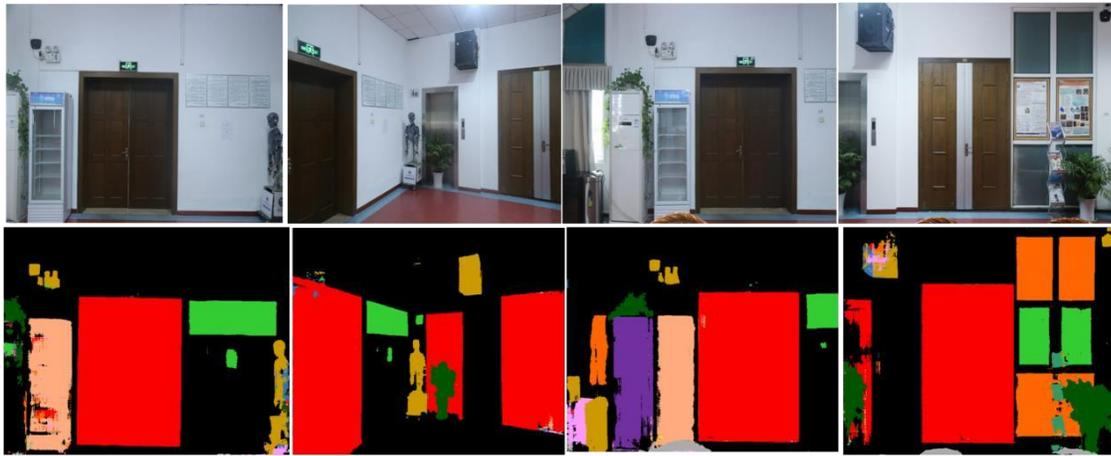
Figure3. 10: the semantic segmentation result of the indoor object obtained by the Deeplabv3+ neural network proposed in this work (a) Test pictures input for the Deeplabv3+ neural network; (b) Semantic segmentation results representing the Deeplabv3+ neural network;
