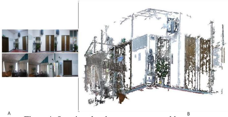
Figure4. 5: point cloud reconstruct a and b
