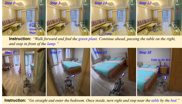
Figure 4. Real-world deployment on a Unitree GO2 quadruped robot. SC 2 -WM enables robust vision-and-language navigation in indoor environments, leveraging internal feedback for self-correction under complex instructions.
