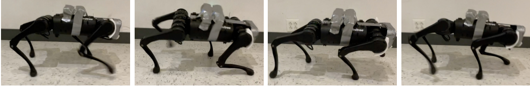
Figure 2: Walking with 1 kg payload (two bottles of 500 ml water are strapped on the back of the robot). The 1 kg payload is out of the normal perturbation of environment parameters used in simulation training shown in Table 1 in the main paper.
